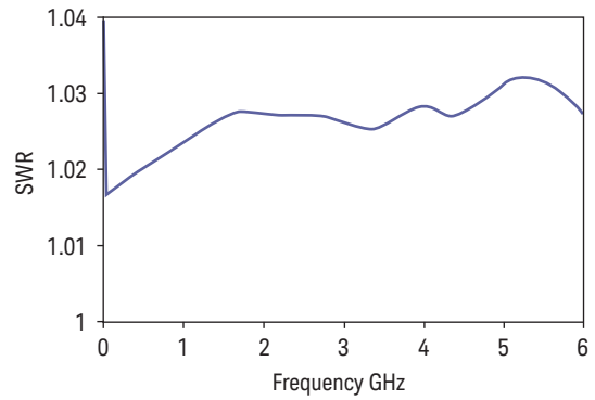
Typical SWR, 100 kHz to 6 GHz (25 ± 10 °C) for N8482A sensor
